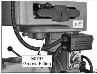
**Figure 54.** Model G0747 headstock gearing grease fitting.
